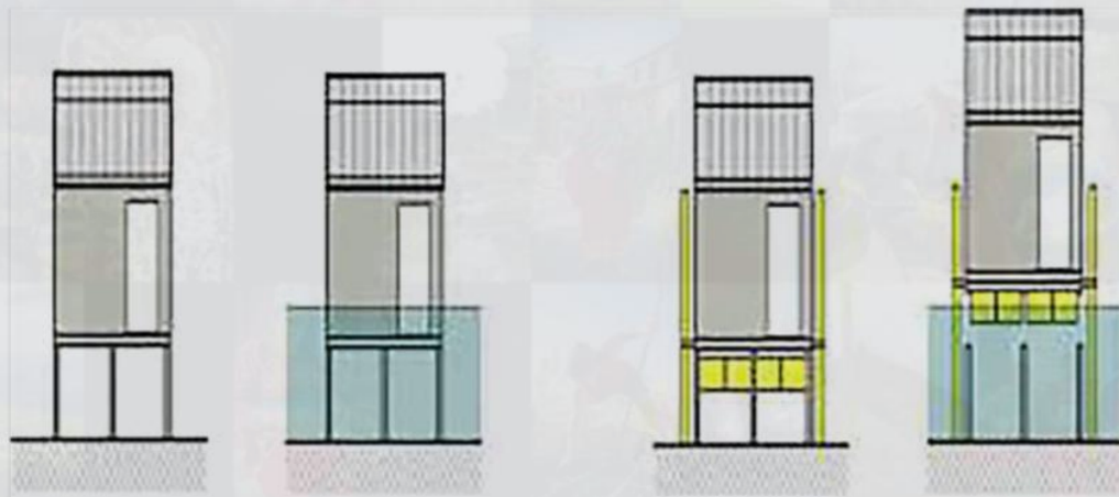
Dwellings on stationary plinths (left, dwelling gets flooded) vs. the amphibious dwelling (right, dwelling floats when flooding occurs) (Image from: Khanolkar, Jadhav, and Patekhede, 2019) 157
